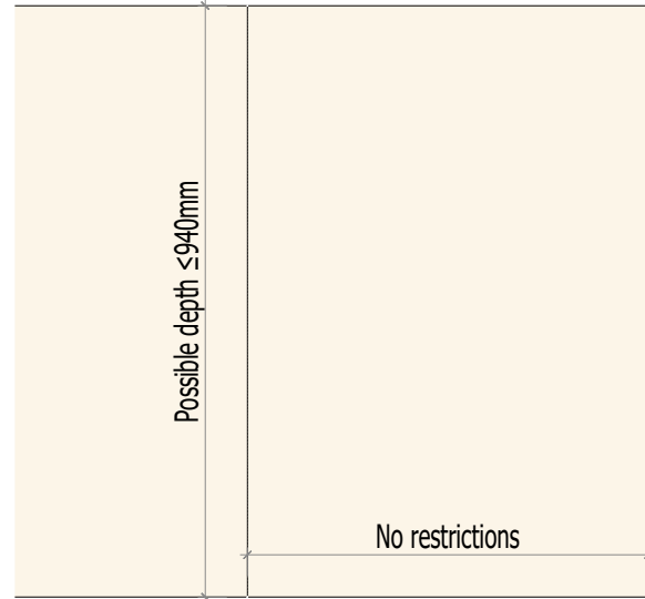
Figure 3 Limitations open slot with horizontal saw and slot cutter (thickness slot \geq 8\text{mm} )
