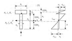
Detailed design of ATC is done using the Euro Code 5 gamma method to calculate stresses and deflections of the individual materials and the effect of the composite action. This method has been verified with extensive structural testing which is available in the appendix if further information is required. Using this framework, the common standards used by design and building professionals can be utilised the same as with typical mass timber or concrete construction.
