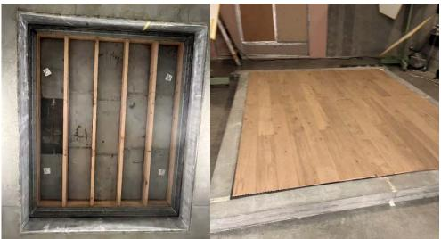
The composite buildup of ATC provides significantly improved acoustic performance compared to timber-only structural solutions, which can prevent the need for further build ups in typical environments. In more sensitive applications such as residential buildings, extensive full scale acoustic insulation testing has been performed in collaboration at CSIRO's laboratory to better understand the airborne and impact acoustic behaviour of ATC panels with acoustic dampening floor build ups.
